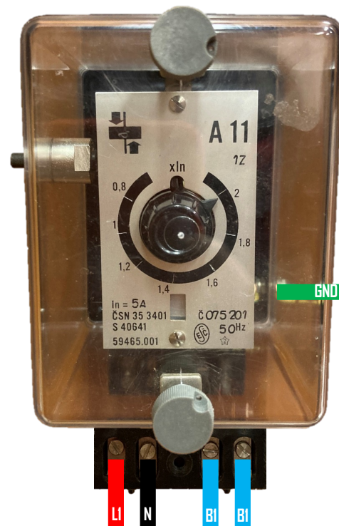
Fig. 13 Overcurrent Relay A11 - testing
